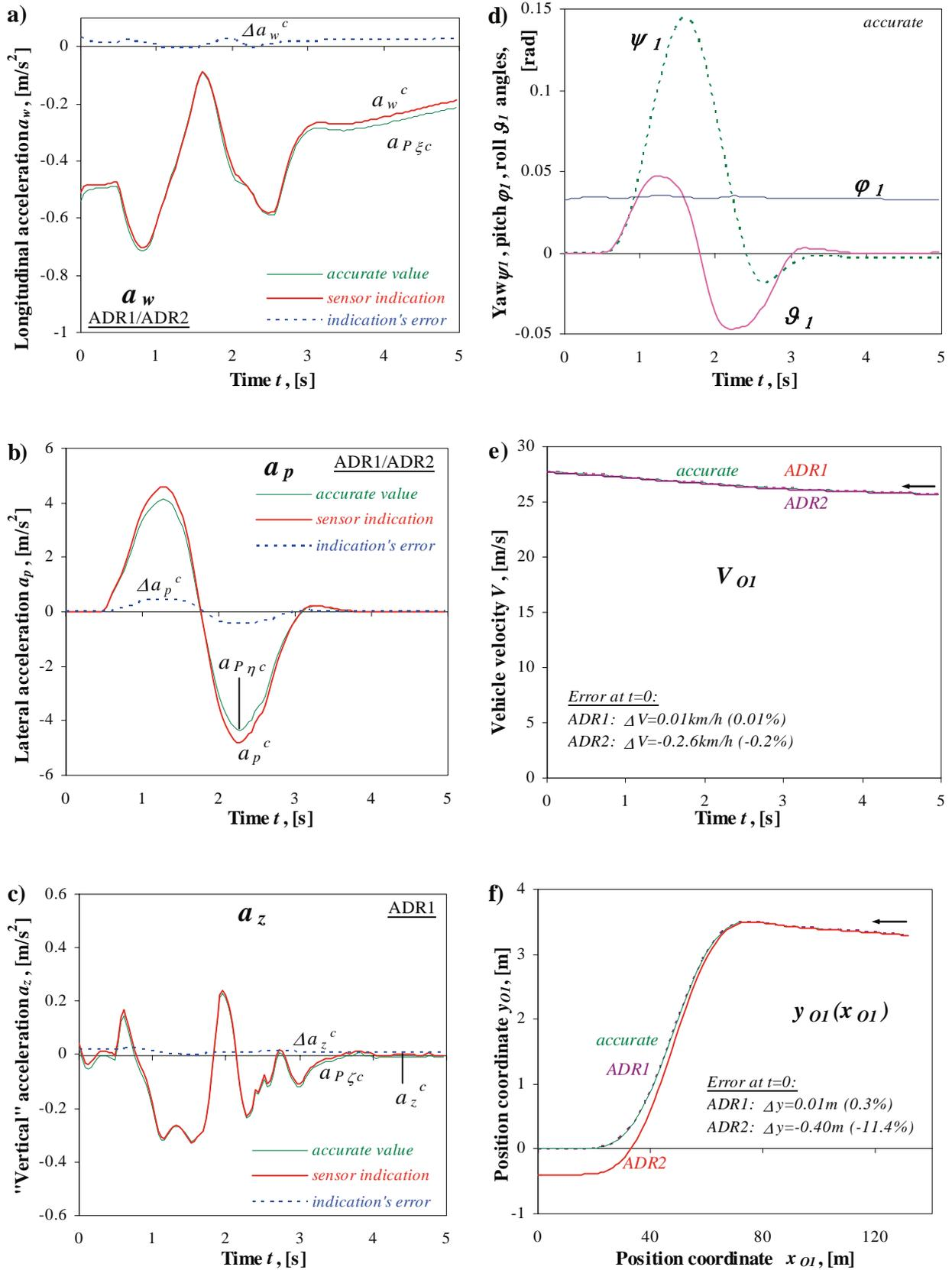
Fig. 9. Singular lane-change maneuver at velocity of  $V_0=100\text{km/h}$ . Time histories of vehicle longitudinal (a), lateral (b) and „vertical“ (c) accelerations: accurate values, sensors indications and their differences – indications errors. Time histories of yaw, pitch and roll angles accurate value (d). The reconstructed velocity of the vehicle (e) and vehicle's C.G. trajectory on the road (f): accurate values and based on ADR1, ADR2 records
