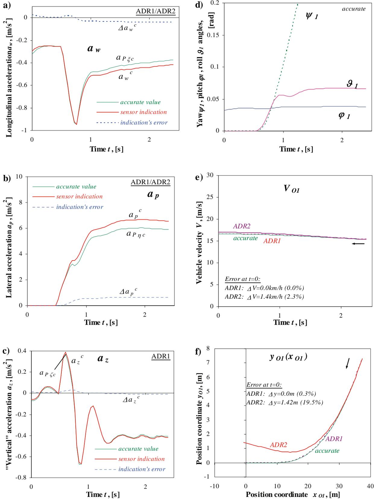
Fig. 10. Turn entering maneuver at velocity of  $V_0=60$ km/h. Time histories of vehicle longitudinal (a), lateral (b) and „vertical“ (c) accelerations: accurate values, sensors indications and their differences – indications errors. Time histories of yaw, pitch and roll angles accurate value (d). The reconstructed velocity of the vehicle (e) and vehicle's C.G. trajectory on the road (f): accurate values and based on ADR1, ADR2 records
