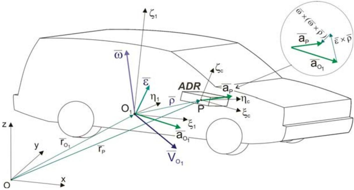
Fig. 3. The model of the kinematics of the movement of the vehicle equipped with an ADR device fixed at point  $P$  ( $r$  – translatory location;  $V$  – translatory movement velocity;  $a$  – translatory movement acceleration;  $\omega$  – angular velocity;  $\varepsilon$  – angular acceleration)
