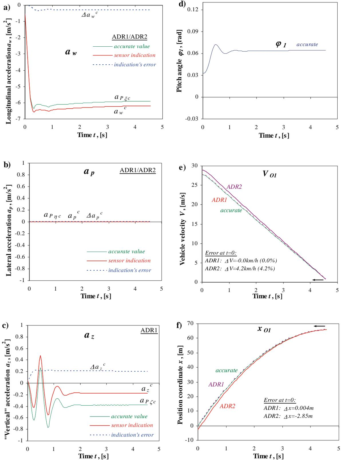
Fig. 8. Straight-line braking from velocity of  $V_0=100\text{km/h}$ . Time histories of vehicle longitudinal (a), lateral (b) and „vertical“ (c) accelerations: accurate values, sensors indications and their differences – indications errors. Time history of pitch angle accurate value (d). The reconstructed velocity of the vehicle (e) and „x“ position on the road (f): accurate values and based on ADR1, ADR2 records
