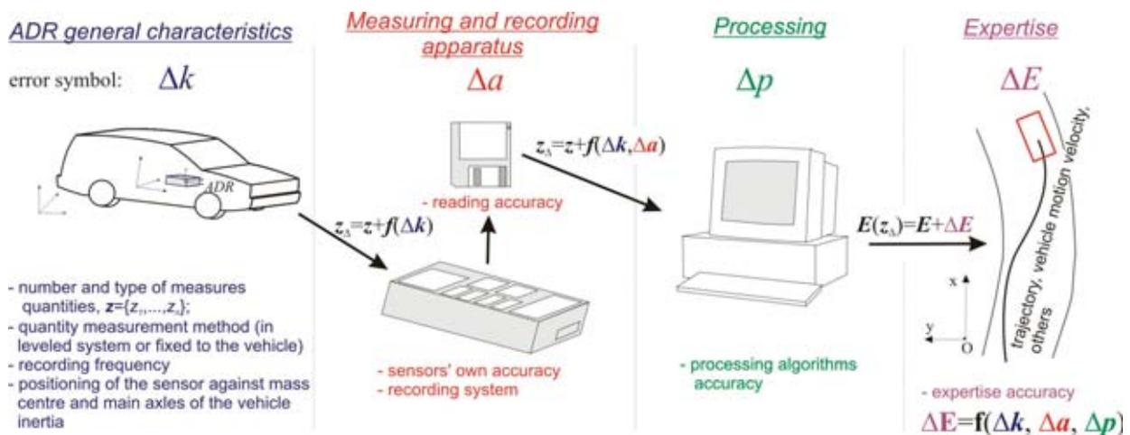
Fig. 1. Sources of errors in vehicle motion reconstruction based on records of ADR devices
