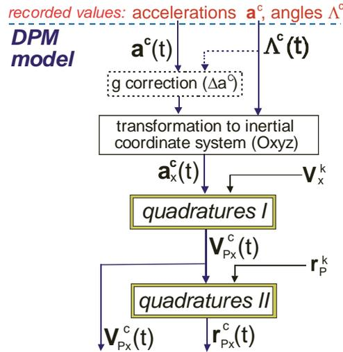
Fig. 6. Block diagram of data elaboration.  $a_x, V_x, r_x$  - vectors of acceleration, velocity and position in the earth-fixed coordinate system Oxyz;  $V^k, r^k$  - final value of velocity and position; index P - denotes the value for point P in which ADR is fixed
