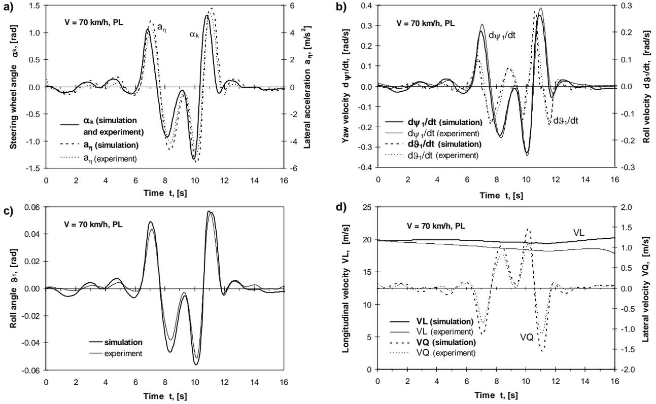
Fig. 7. Double lane - change maneuver. Comparison of selected time histories of sensors indications in the experiment and in the simulation (ZL3DSYM plus ADR): a) the vehicle lateral acceleration, b) yaw velocity  $d\psi_1/dt$  and roll angular velocity  $d\theta_1/dt$ , c) roll angle  $\theta_1$ , d) vehicle longitudinal velocity VL and lateral velocity VQ (only ZL3DSYM). Partially loaded vehicle (PL)
