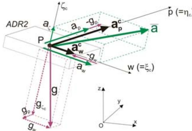
Fig. 5. Graphical interpretation of the readings of the sensors measuring the longitudinal and the lateral accelerations (example for ADR2 type device)
