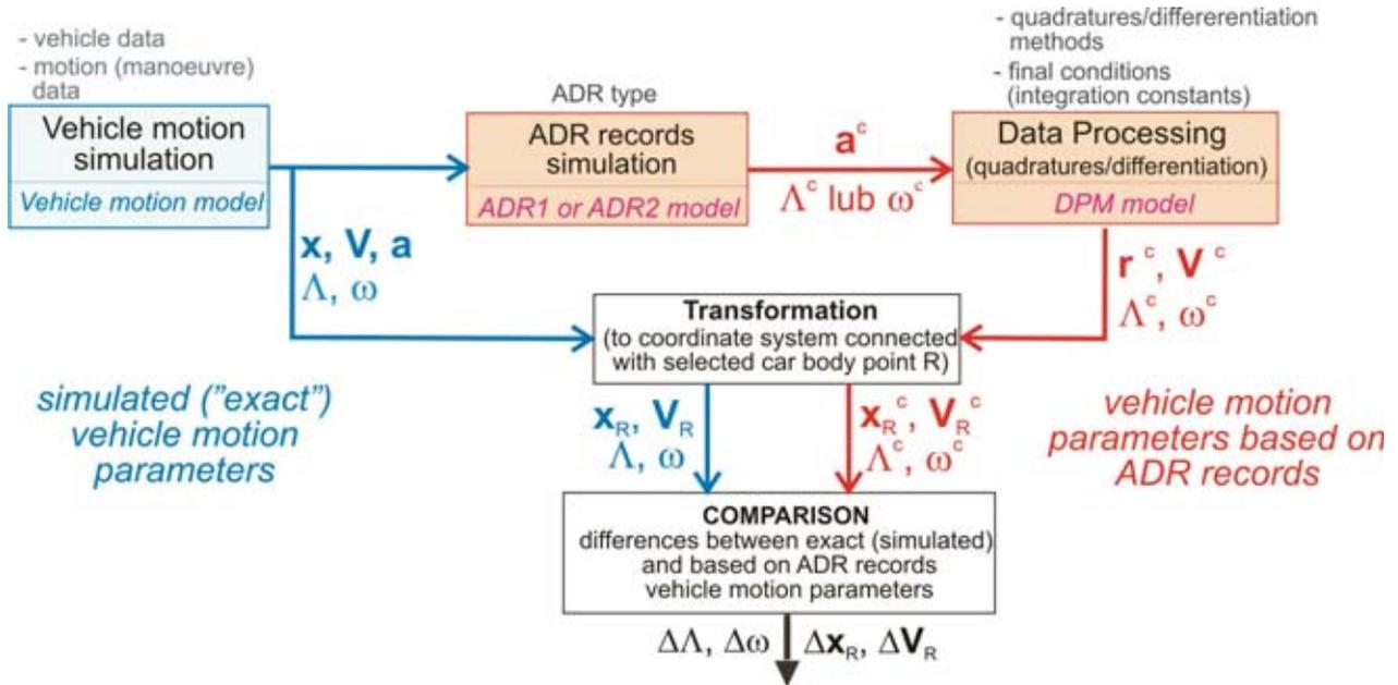
Fig. 2. Motion reconstruction accuracy assessment method based on ADR devices records:  $a, V, \omega, r, \Lambda$  – components vectors (respectively): acceleration, velocity, angular velocity, position, angles
