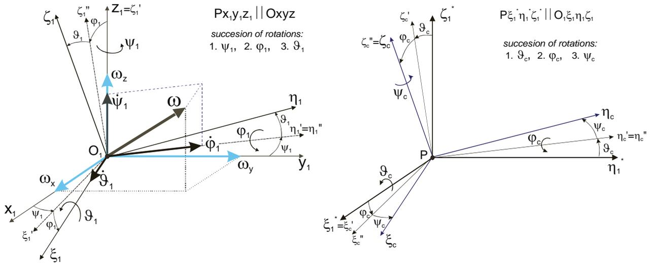
Fig. 4. The angular positioning of the coordinate systems:  $O_1\xi_1\eta_1\zeta_1$  in relation to  $Oxyz$  and  $P\xi_c\eta_c\zeta_c$  in relation to  $O_1\xi_1\eta_1\zeta_1$
